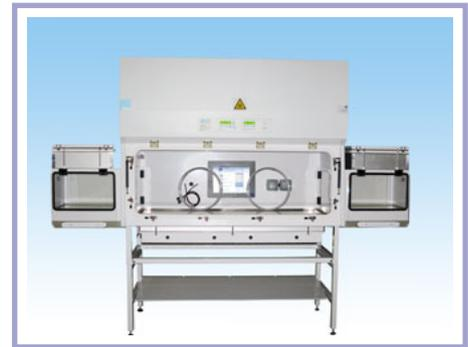
Envair responded initially by building several isolators with LCD monitors mounted in the rear wall to allow operators to access information, but not to input information or to respond to requests. This limitation was then overcome by sourcing and installing suitable LCD touchscreen monitors which allowed operators to feed information back in real time.
